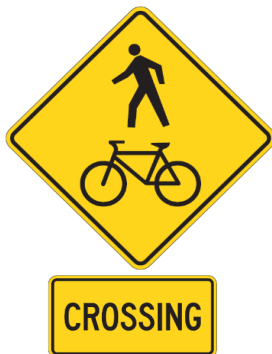
Figure 47. Pedestrian and bicycle crossing ahead (Wc-15) above and crossing warning tab (Wc-32t) below (Ontario Ministry of Transportation).
