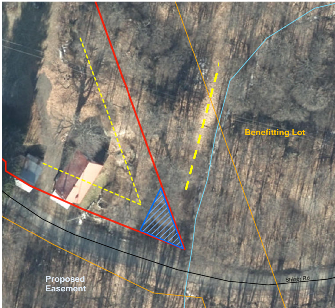
Figure 2: Air photo showing the subject property, lot line setbacks, the proposed easement and the benefiting lot. The seven metre lot line setbacks are shown with the yellow dashed line, the proposed easement is shown in blue hatching.
