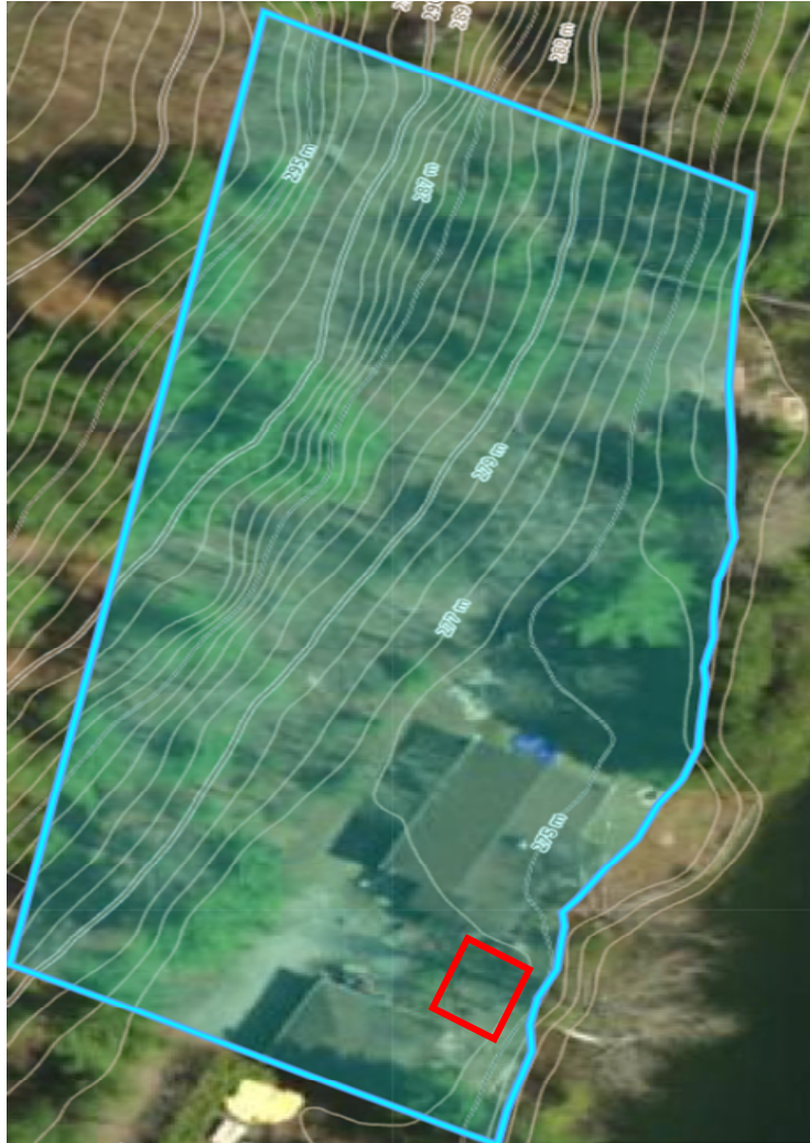
Figure 1. One-metre elevation contour map of the subject property with the proposed development location outlined in red. Larger spacing between contour lines indicate flatter terrain.
