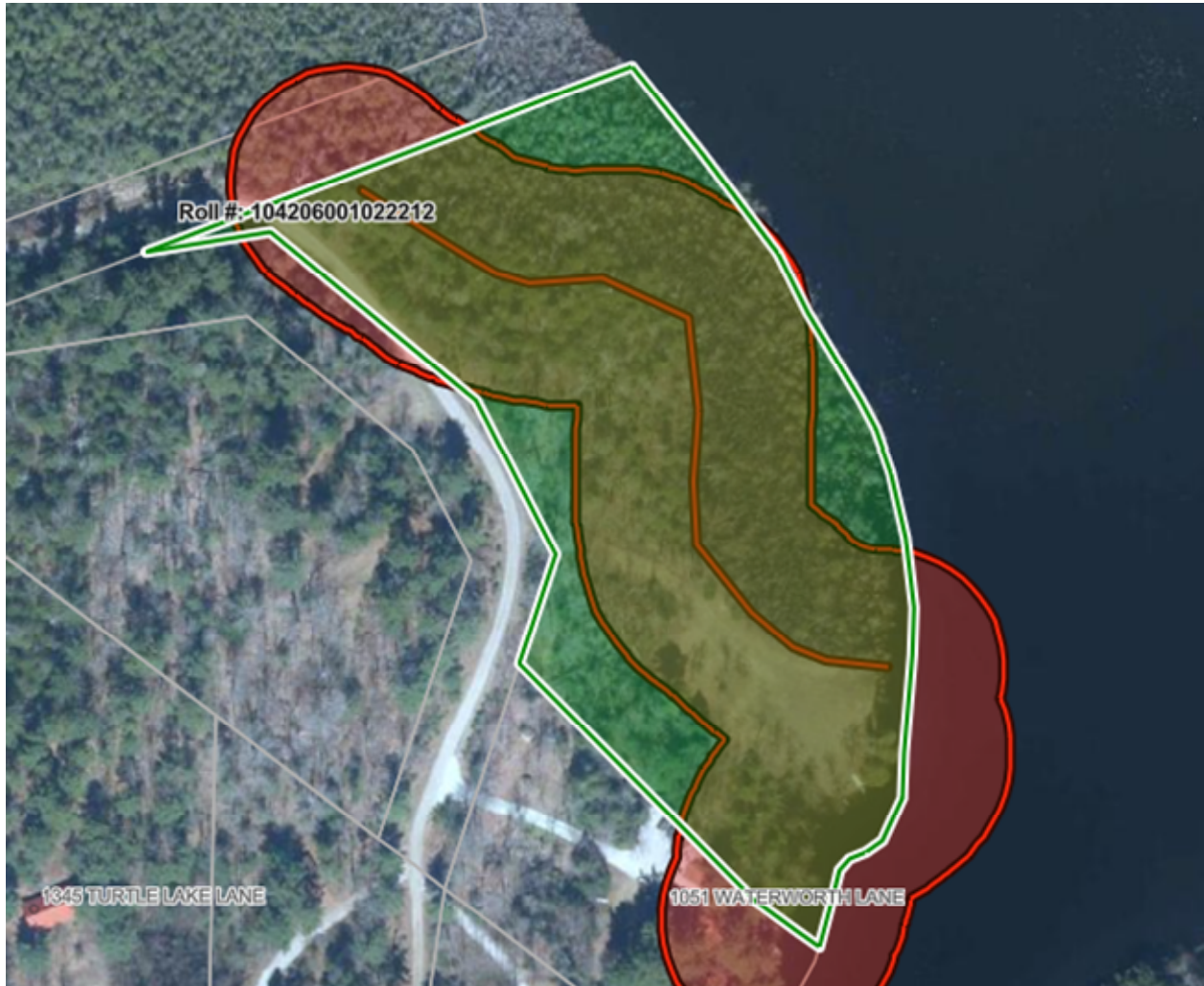
Figure 1. Image of the subject property showing the approximate edge of wetland with a 30 metre (98.4 foot) setback applied to both the wetland edge and the shoreline.
