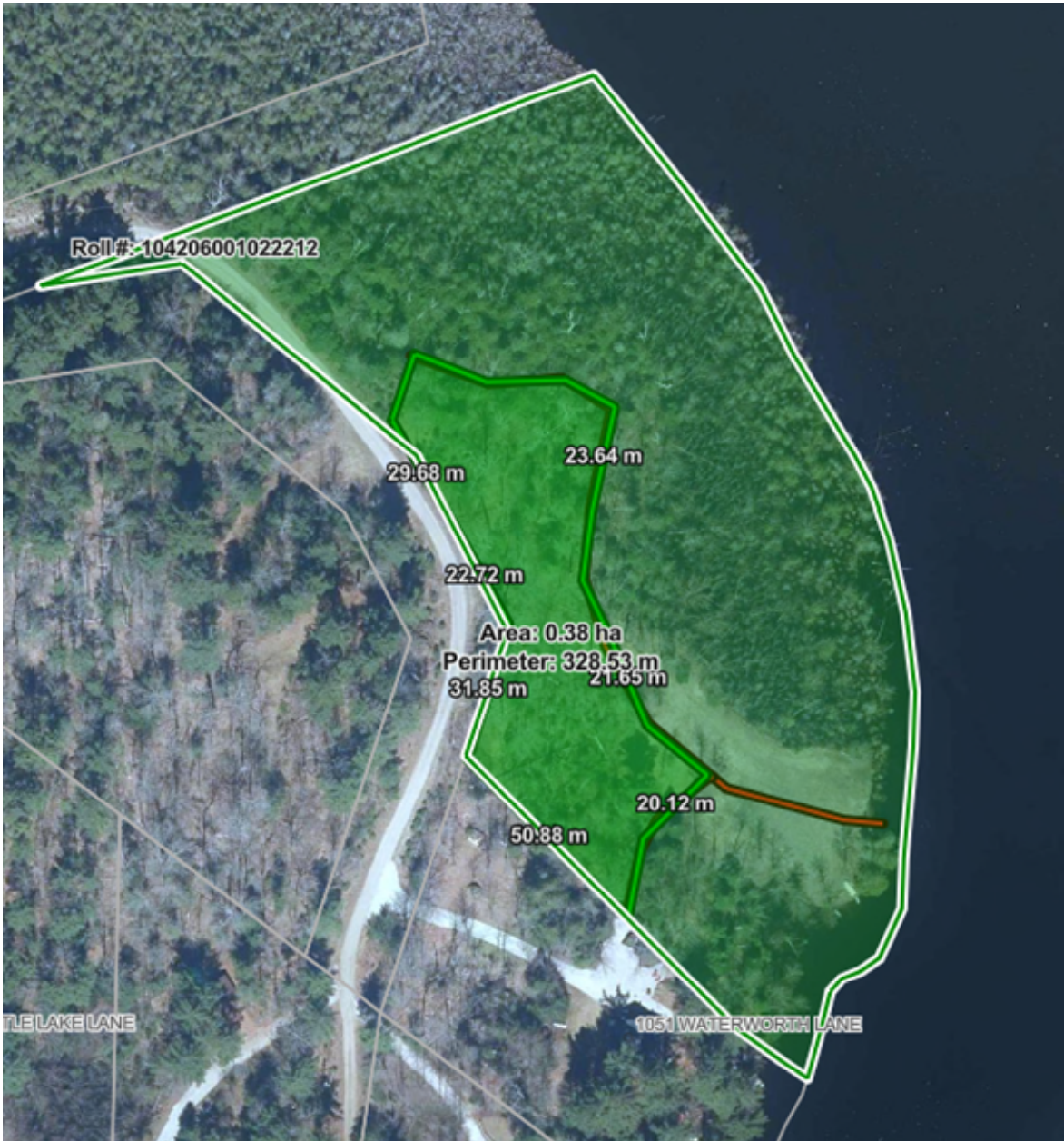
Figure 2. An aerial image of the subject lot showing the development envelope when the setback is 15 metres (49.2 feet) from the wetland and 30 metres (98.4 feet) from the shoreline.
