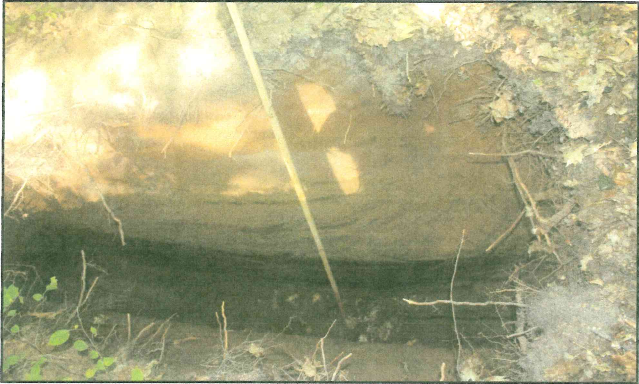
Photograph 9 – Native Soil Depth of 3m Confirmed at Septic Envelope Site (September 26, 2017)
