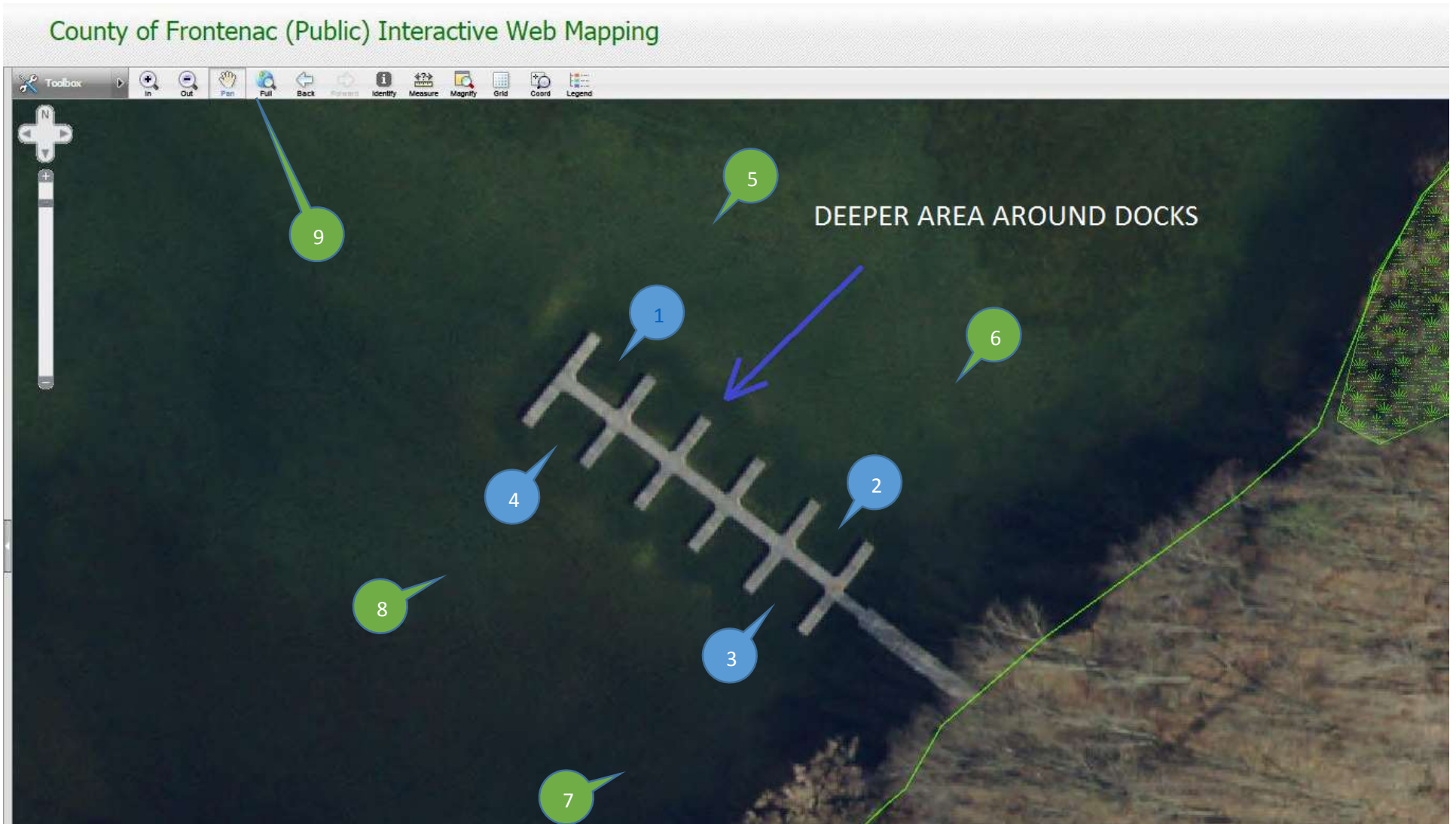
Figure 2. Applewood Subdivision 22 Slip Dock - 200ft long dock in 1ft of water
