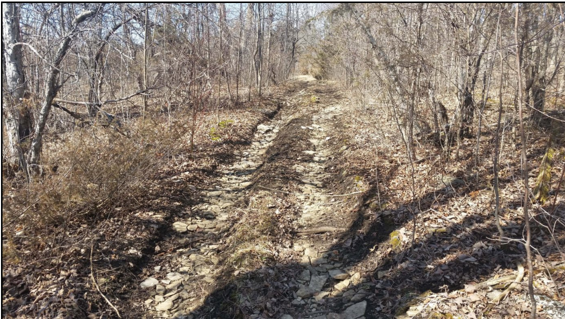
Plate 1: Shallow topsoil cover towards the southern end of the proposed Phase 1 development. Less than 10 centimetres of topsoil is present in this area. The track has eroded through the topsoil to expose the bedrock surface.
